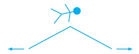
The step-ladder needs something to hold the two sides of the ladder together if it is not to collapse when weight is put onto it.
